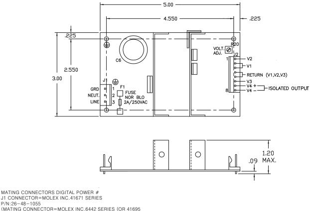
J1 CONNECTOR=MOLEX INC.41671 SERIES P/N:26-48-1055 (MATING CONNECTOR=MOLEX INC.6442 SERIES (OR 41695 SERIES) J2 CONNECTOR=MOLEX INC. 41671 SERIES P/N:26-48-1085 (MATING CONNECTOR=MOLEX INC.6442 SERIES (OR 41695 SERIES) P/N:26-03-4081 (OR 09-50-8081) (MATING CRIMP TERMINALS=MOLEX INC.6838 SERIES, P/ N:08-52-0113 OR 08-52-0112)
