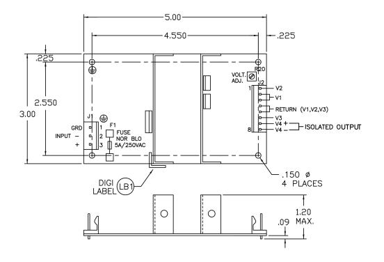
MATING CONNECTORS DIGITAL POWER # J1 CONNECTOR=MOLEX INC.41671 SERIES P/N:26-48-1055 (MATING CONNECTOR=MOLEX INC.6442 SERIES (OR 41695 SERIES)
